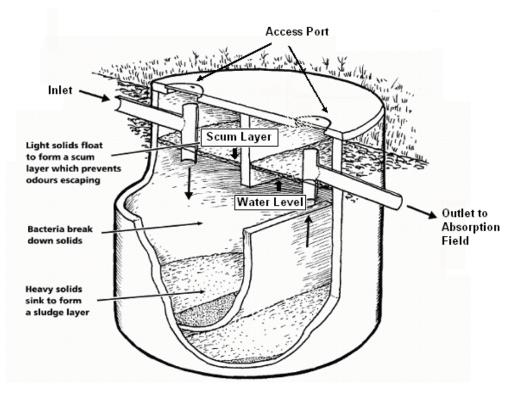
The standard septic tank in some ways is like a big stomach. It is fed through an inlet pipe with **sewage** from the toilet and **greywater** from the washing machine, kitchen sink and bathroom. What goes into the tank is usually a mixture of human waste, water, washing detergents, chemicals and other materials. This wastewater is digested by a host of different bacteria. When the septic tank gets too full, some of the wastewater flows out of the primary tank to the holding well.
