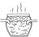
house flows into a septic tank, where solids, fats and greases separate from the effluent which then flows into a holding well. Tankers collect effluent from this holding well on a fortnightly basis or more frequently for larger houses.
