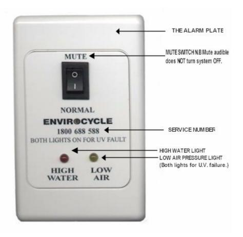
Bellow is a picture of the *ENVIROCYCLE Chlorine Disinfection Model* 14 Alarm Plate and Control Box.
