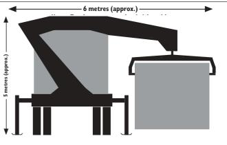
Truck Crane - Unloading (rear view) Note: Truck unloads to rear, but crane may traverse either side (see diagram below).
