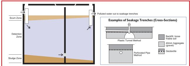
A simplified cross-section of a septic tank, showing how solid matter is separated and retained, by floating (scum) or settling (sludge), as the water passes slowly through. Sludge and scum gradually build up over time and must be pumped out. The wastewater which flows out of the tank is partially treated (most of the solids removed) but still heavily contaminated.
