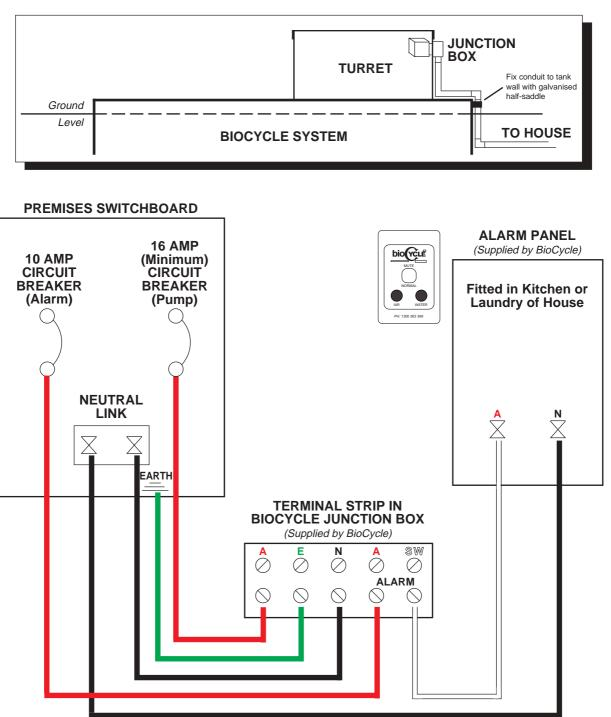
**IMPORTANT NOTE: DO NOT** feed the system with one circuit and loop the two active terminals. If you only use one circuit to feed the system, under fault conditions the whole system will shut down and the alarm will not operate.
