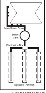
Typical soakage trench configurations for different block sizes (NOTE: Not to scale. Actual design dependent on local regulations)
