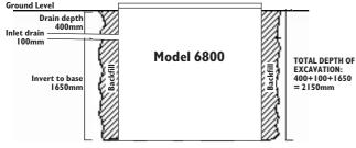
If the inlet drain must be so deep that the top lip of the tank will be below ground level, Riser(s) must be added (see further explanation and illustration at right).
