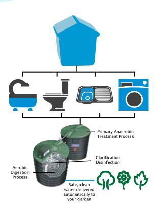
The Aqua-nova® Treatment Process Separates, Treats, Clarifies, Sanitises, Irrigates
