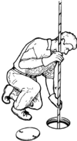
3) Withdraw it completely, noticing the size and position of the scum mark and the depth of the sludge.
