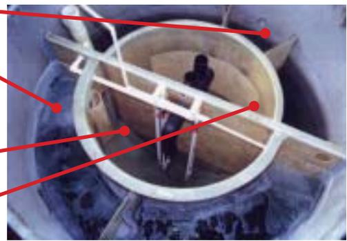
Note: Most current standard BioCycle models have a concrete centre wall.
